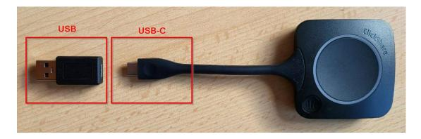
At the end of the dongle there is an adapter from USB-C to USB, which can be plugged in or removed as required.
