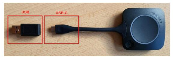
At the end of the dongle there is an adapter from USB-C to USB, which can be plugged in or removed as required.
